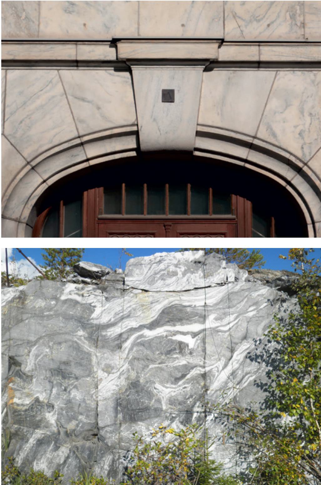
Figure 29. Various appearances of the Ruskeala marble A. Façade of the Helsingin Säästöpankki building in Helsinki. B. The "Italian quarry" in Ruskeala. Photos: A. Paavo Härmä, B. Andrei Ivanov.
