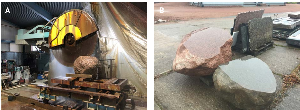
Figure 2. A. Manufacturing of rhyme stones at the processing plant of the company Vikmanin Kivi Ky. B. Half-finished rhyme stones, only missing the rhymes. Photos: Olavi Selonen.
