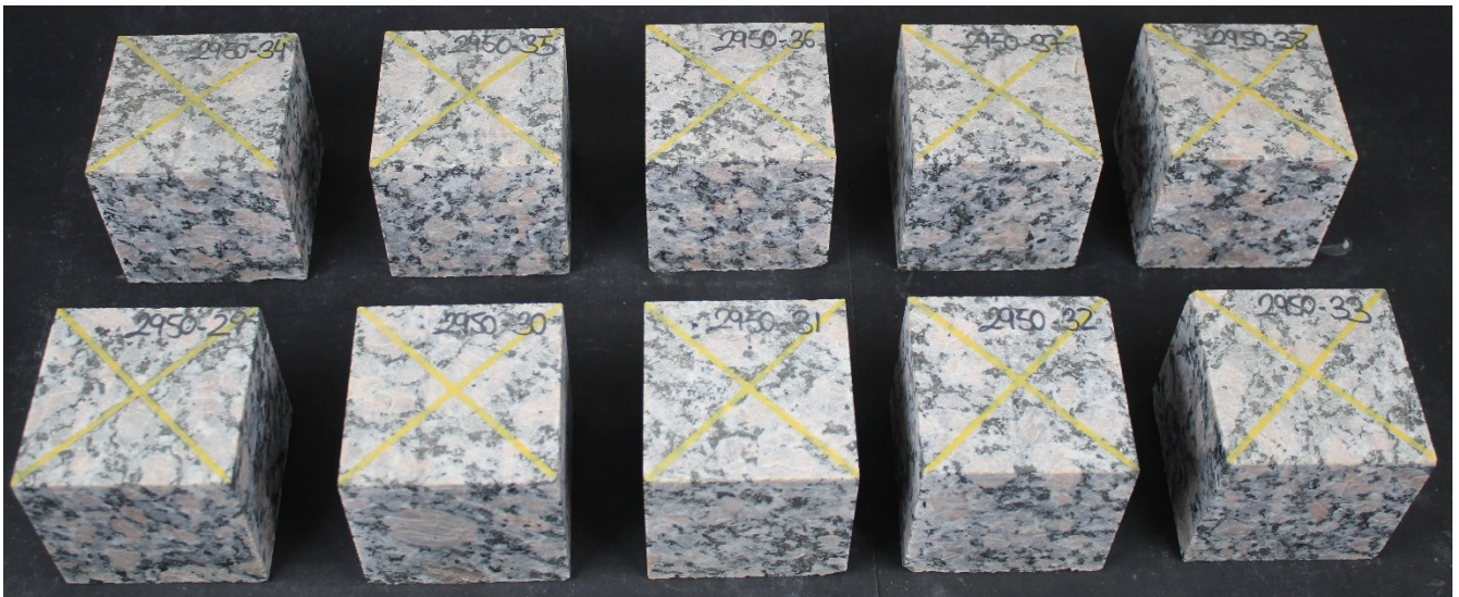
Set 2 after 56 freeze-thaw cycles
