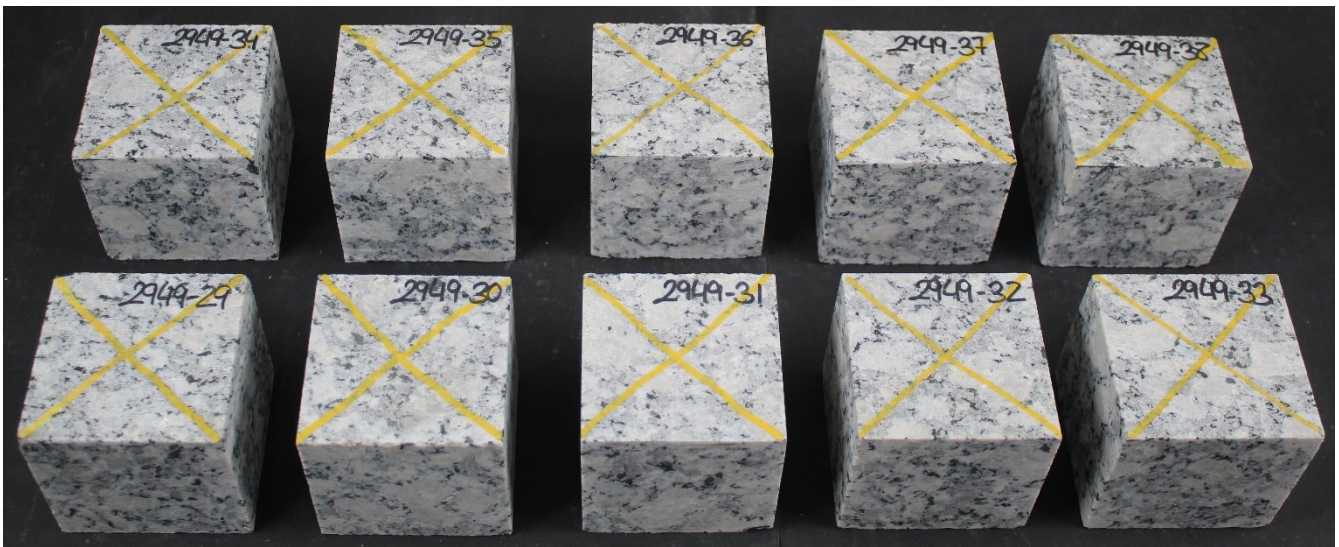
Set 2 after 56 freeze-thaw cycles
