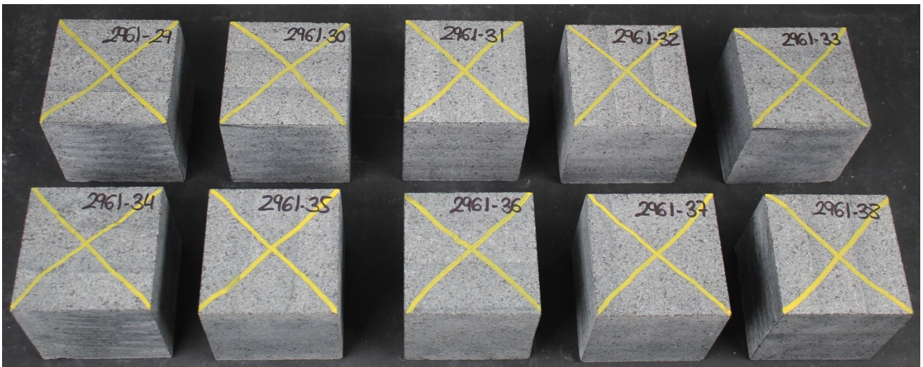
Set 2 after 56 freeze-thaw cycles
