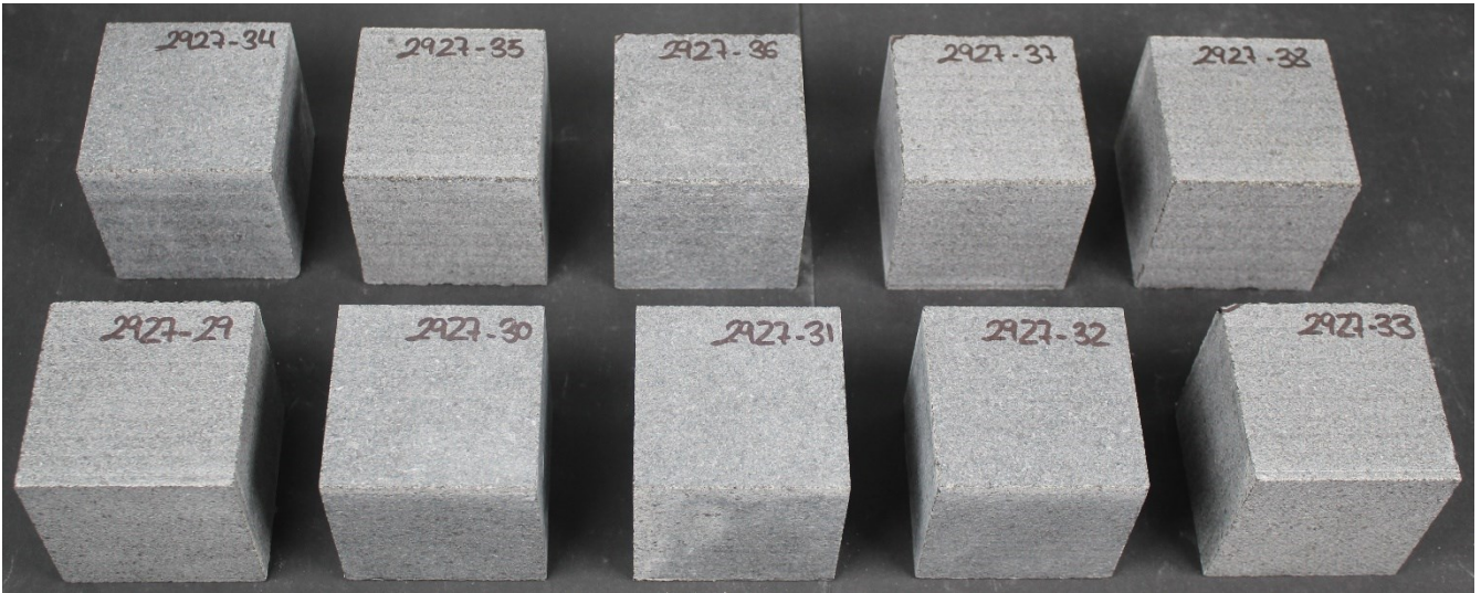
Set 2 after 56 freeze-thaw cycles
