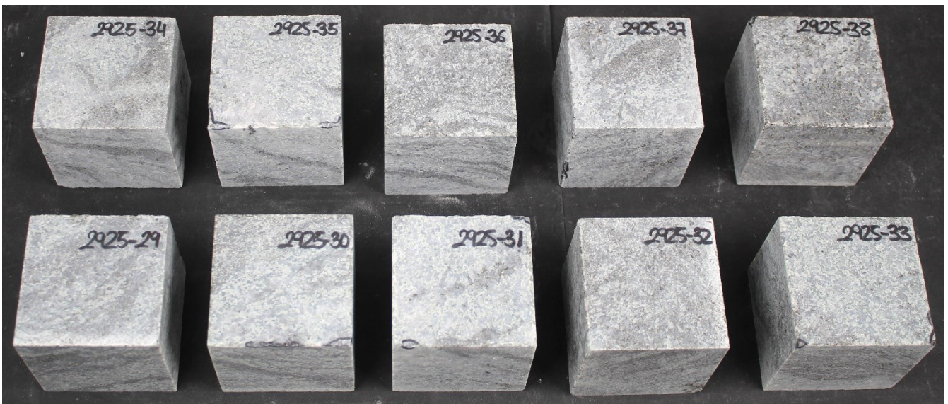
Set 2 after 56 freeze-thaw cycles
