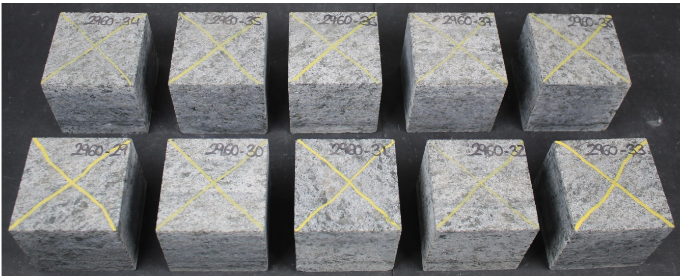
Set 2 after 56 freeze-thaw cycles
