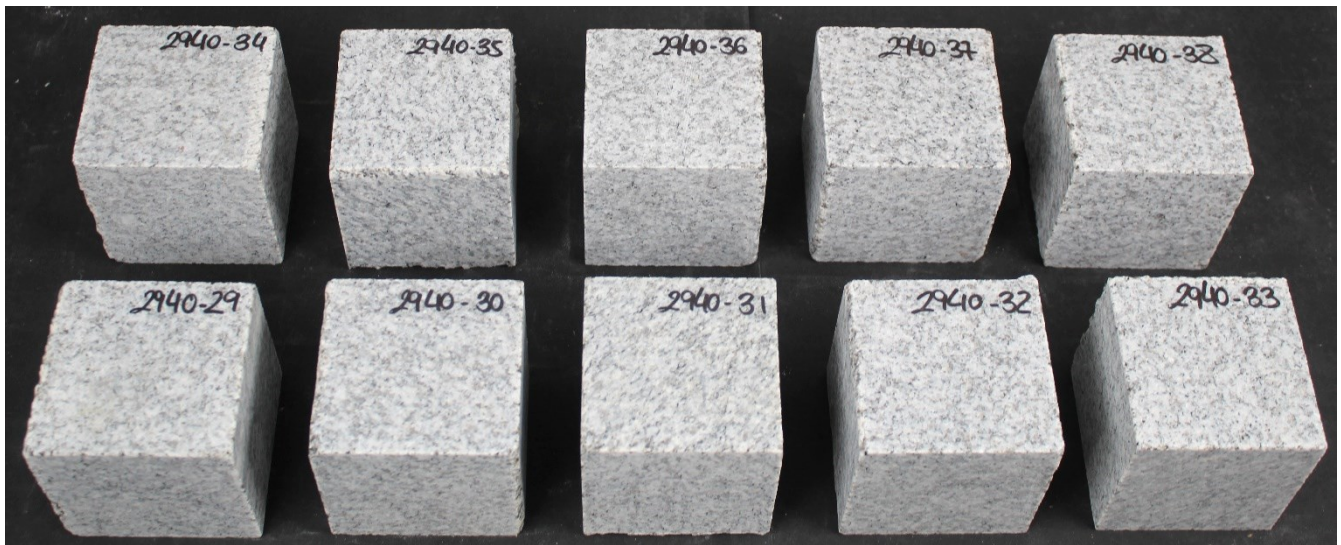
Set 2 after 56 freeze-thaw cycles
