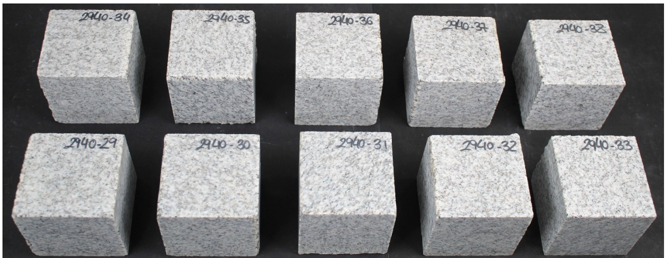
Set 2 after 56 freeze-thaw cycles
