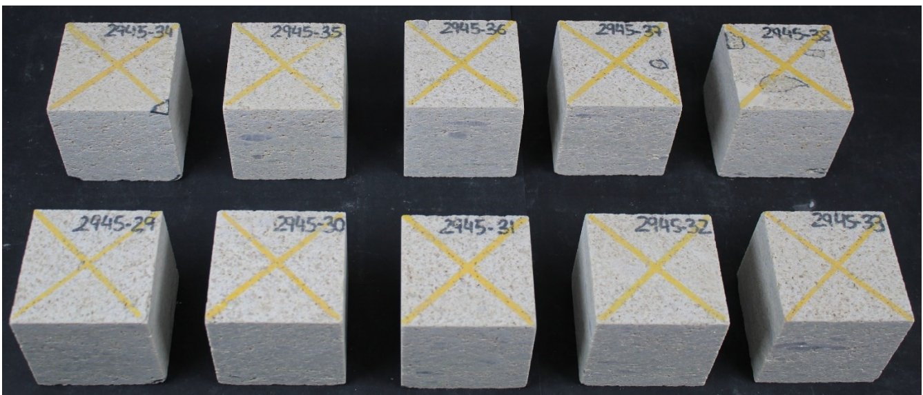
Set 2 after 56 freeze-thaw cycles
