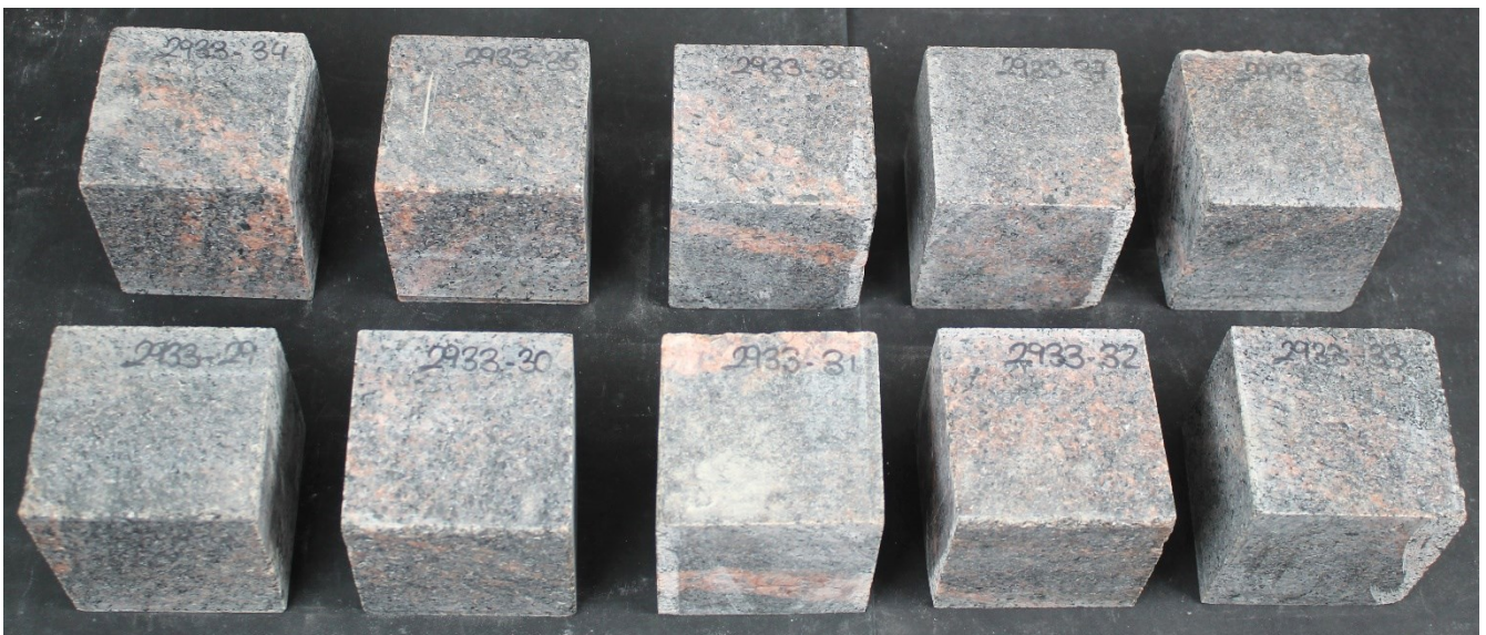
Set 2 after 56 freeze-thaw cycles
