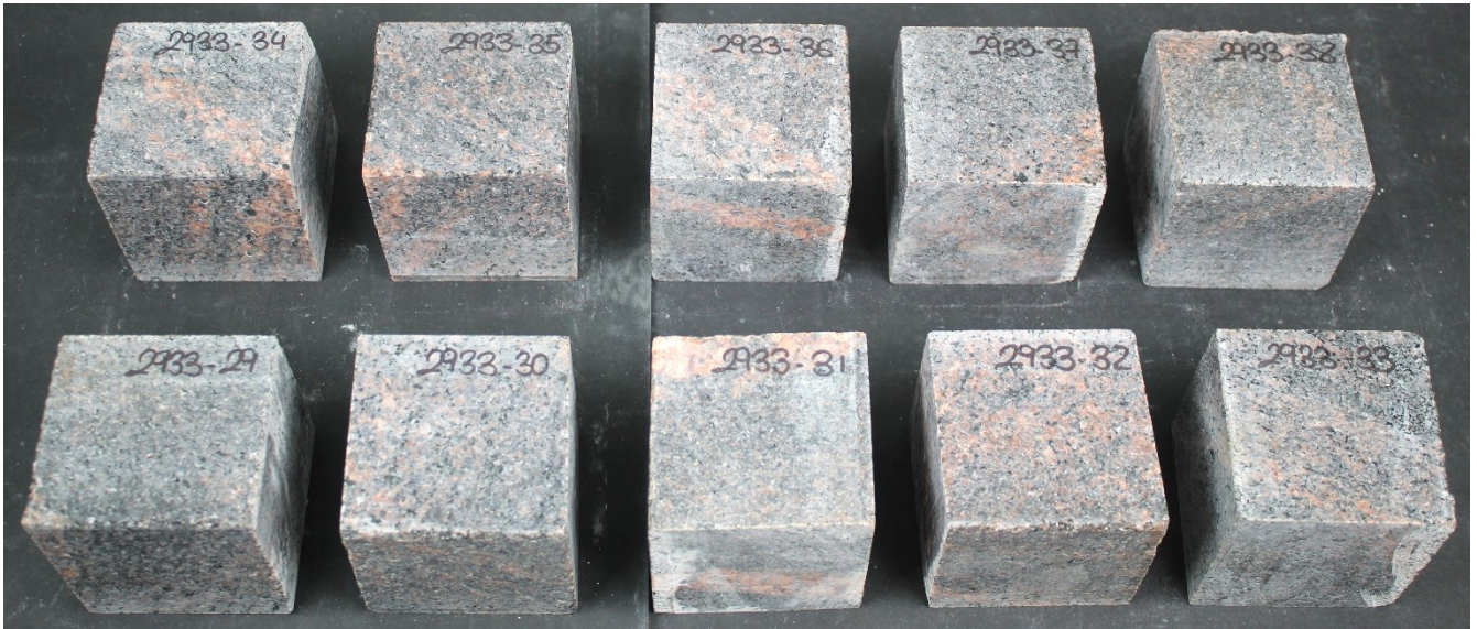
Set 2 after 56 freeze-thaw cycles
