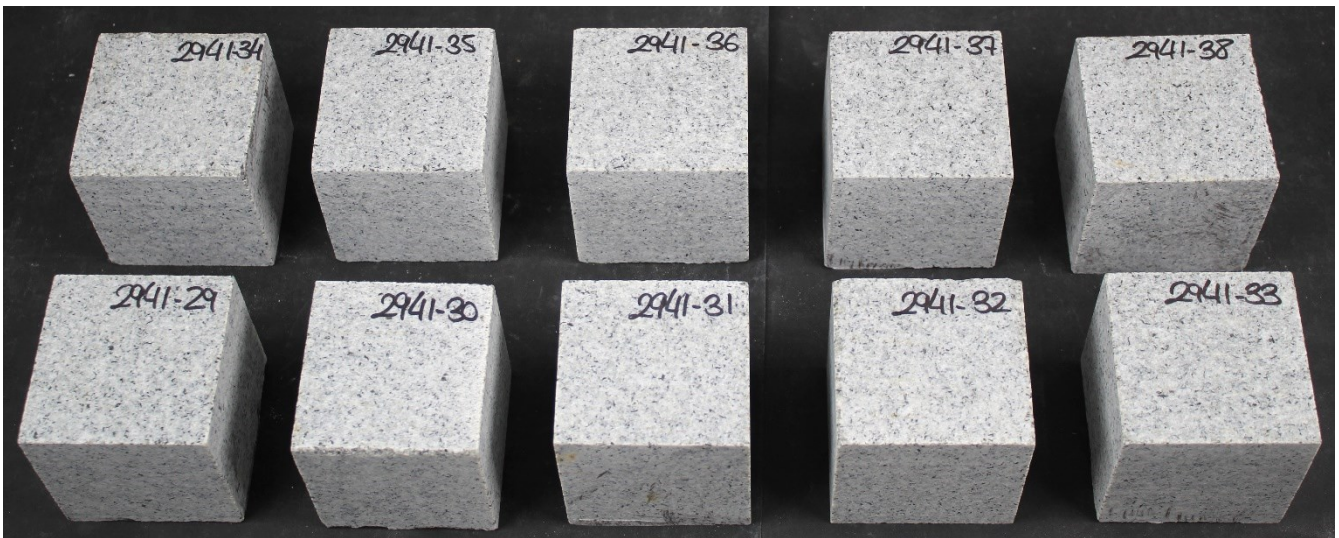
Set 2 after 56 freeze-thaw cycles
