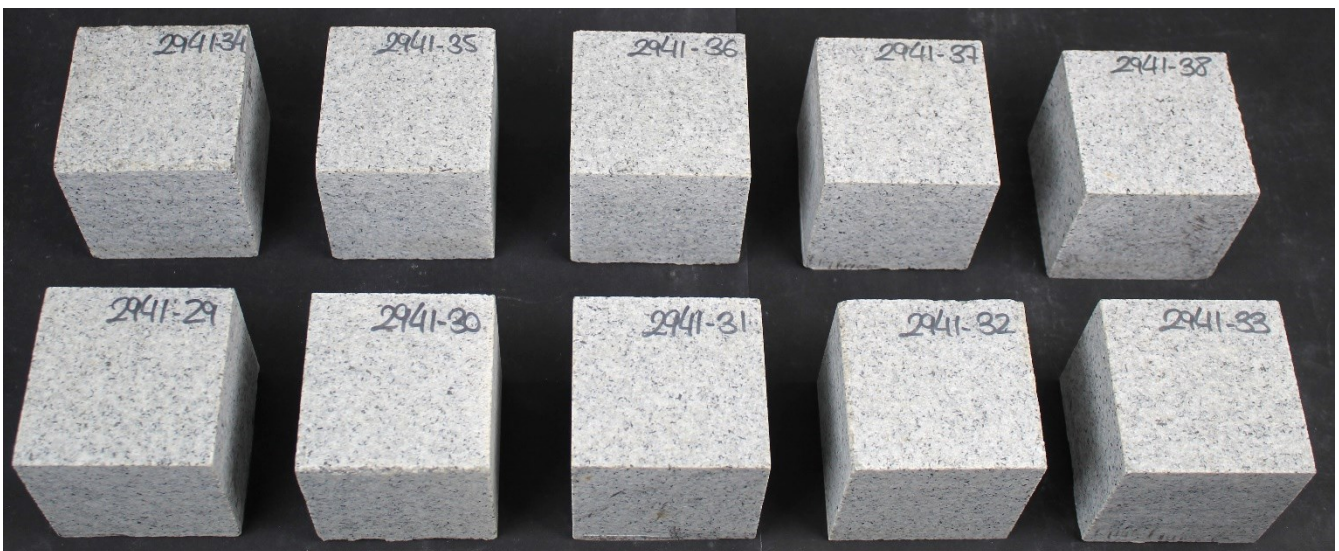
Set 2 after 56 freeze-thaw cycles
