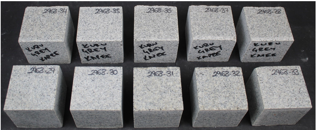
Set 2 after 56 freeze-thaw cycles
