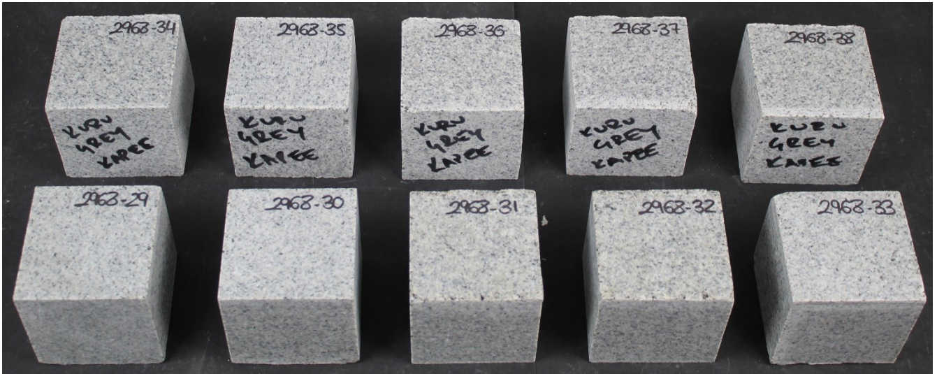
Set 2 after 56 freeze-thaw cycles
