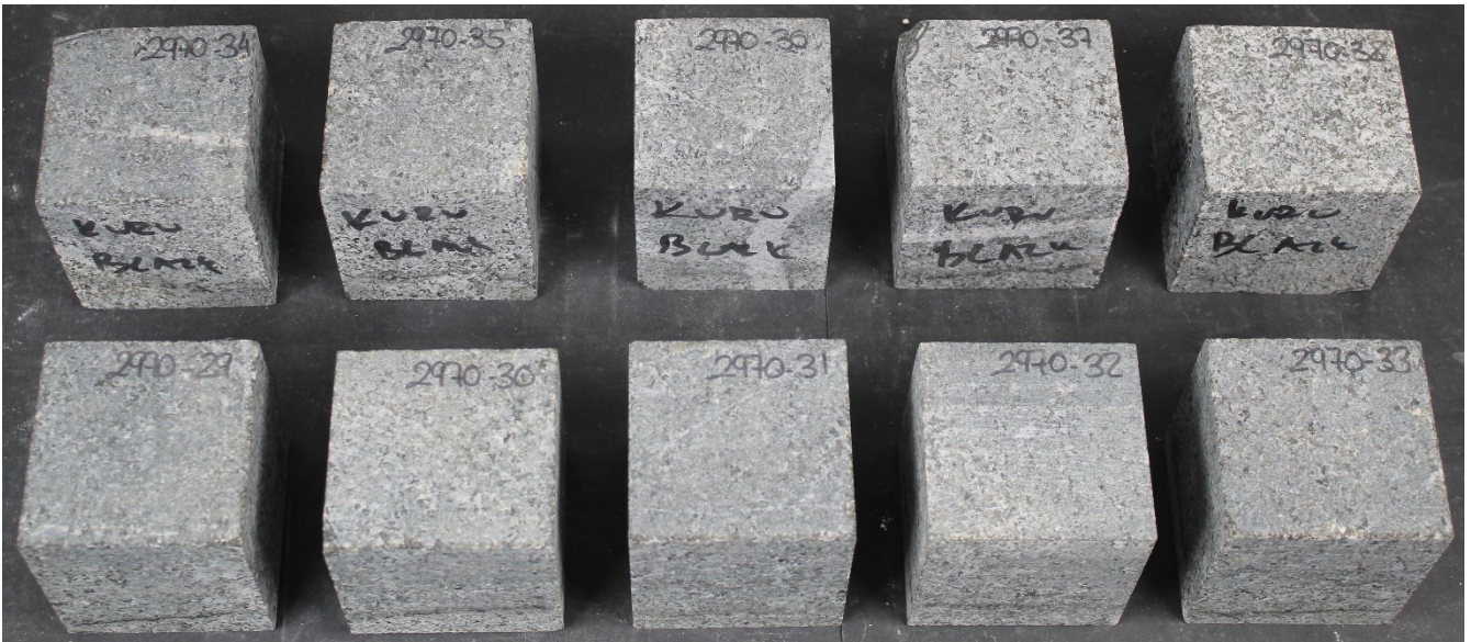
Set 2 after 56 freeze-thaw cycles
