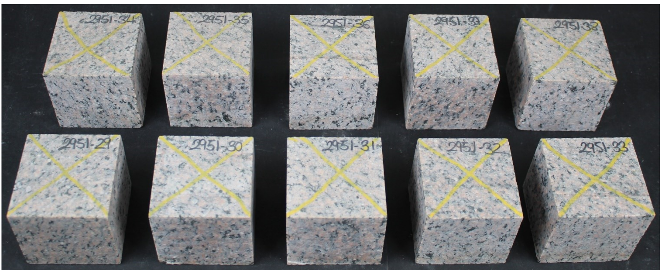
Set 2 after 56 freeze-thaw cycles
