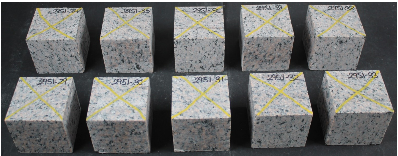
Set 2 after 56 freeze-thaw cycles
