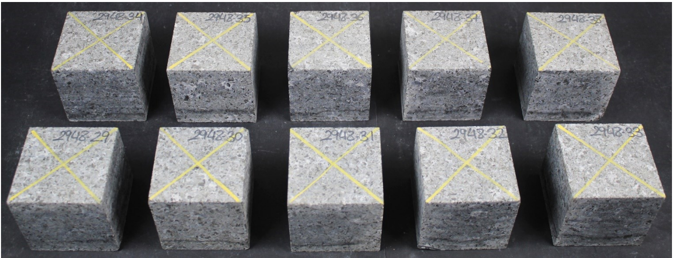
Set 2 after 56 freeze-thaw cycles
