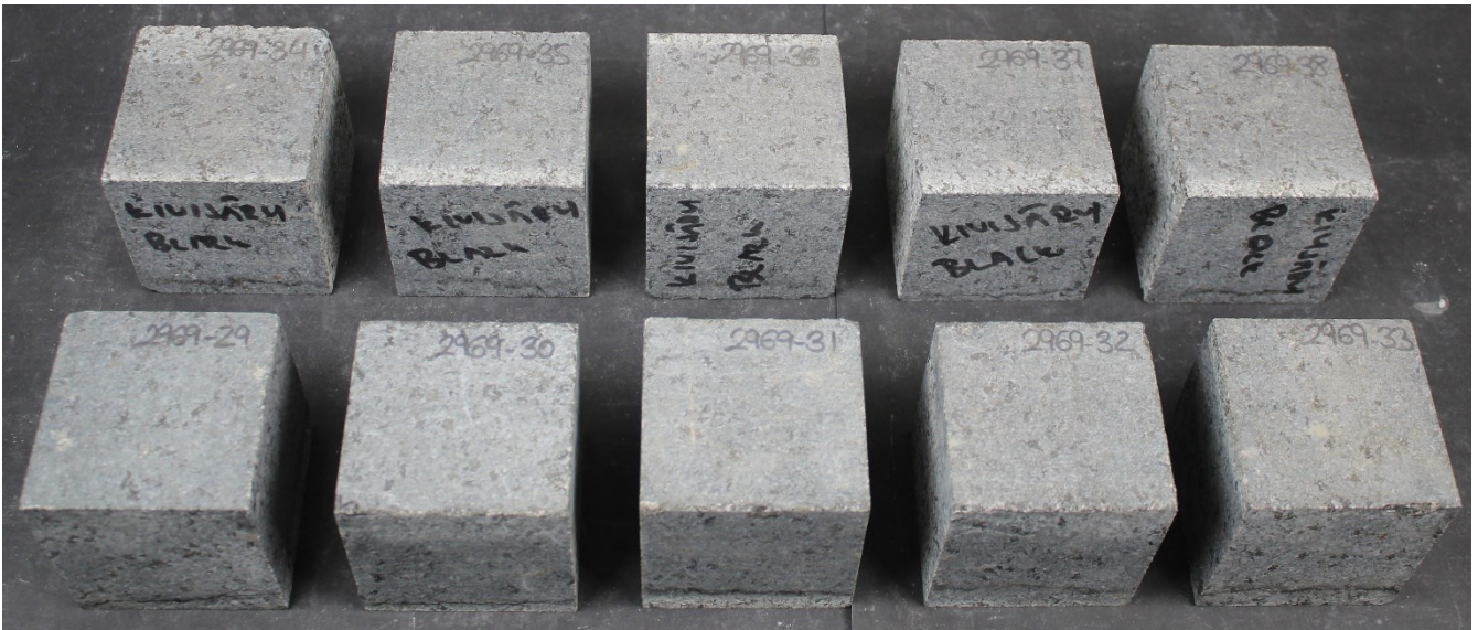
Set 2 after 56 freeze-thaw cycles
