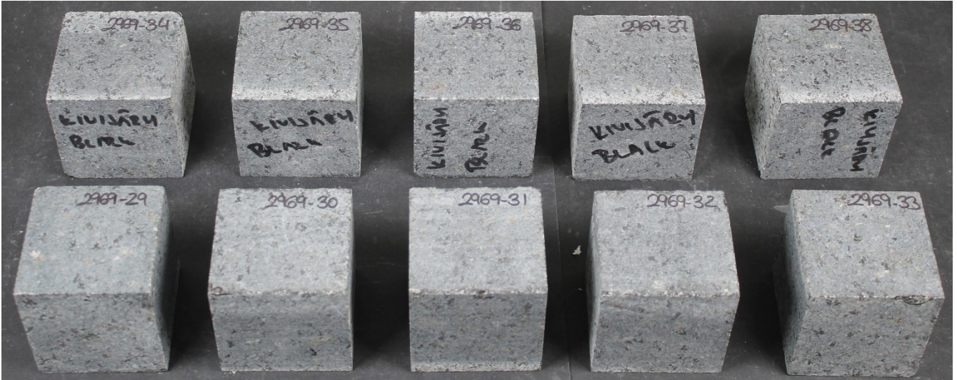
Set 2 after 56 freeze-thaw cycles
