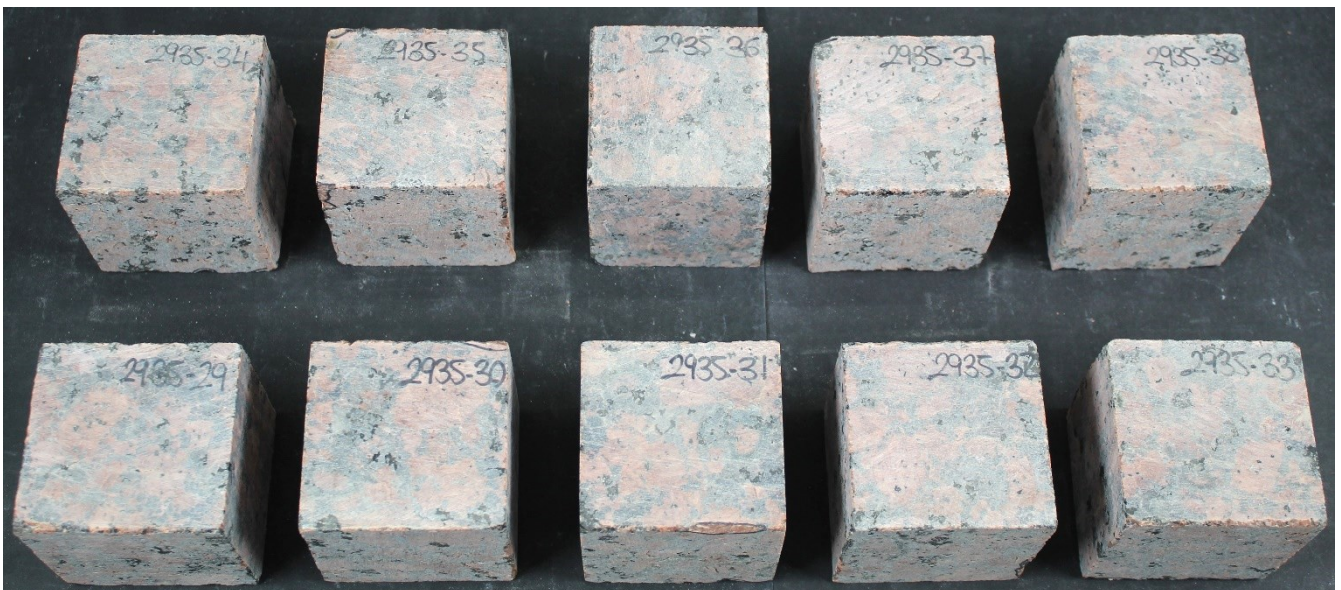
Set 2 after 56 freeze-thaw cycles
