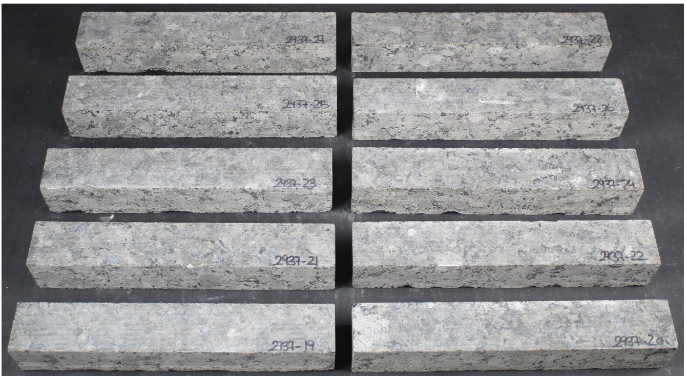
Set 2 after 56 freeze-thaw cycles
