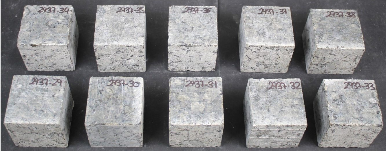
Set 2 after 56 freeze-thaw cycles
