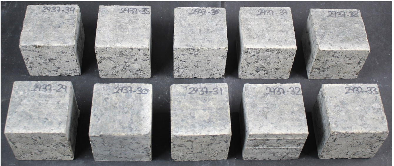
Set 2 after 56 freeze-thaw cycles
