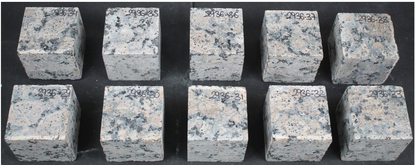
Set 2 after 56 freeze-thaw cycles
