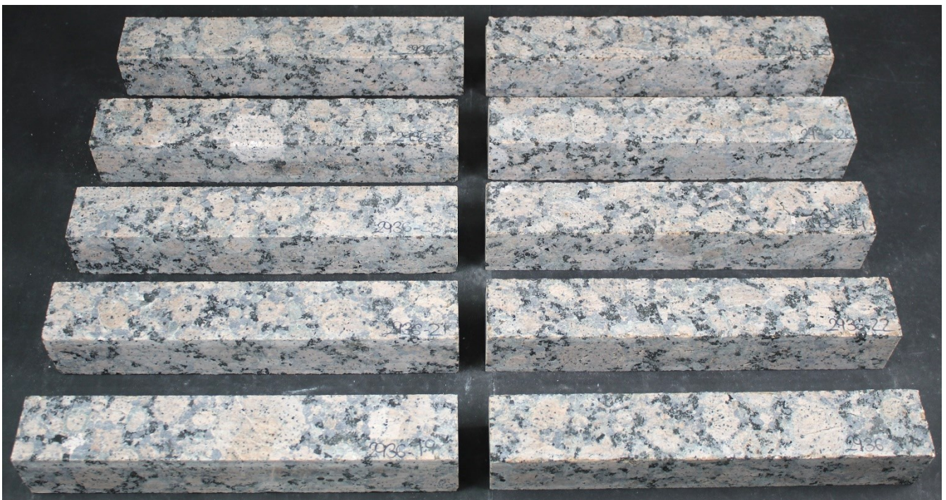
Set 2 after 56 freeze-thaw cycles
