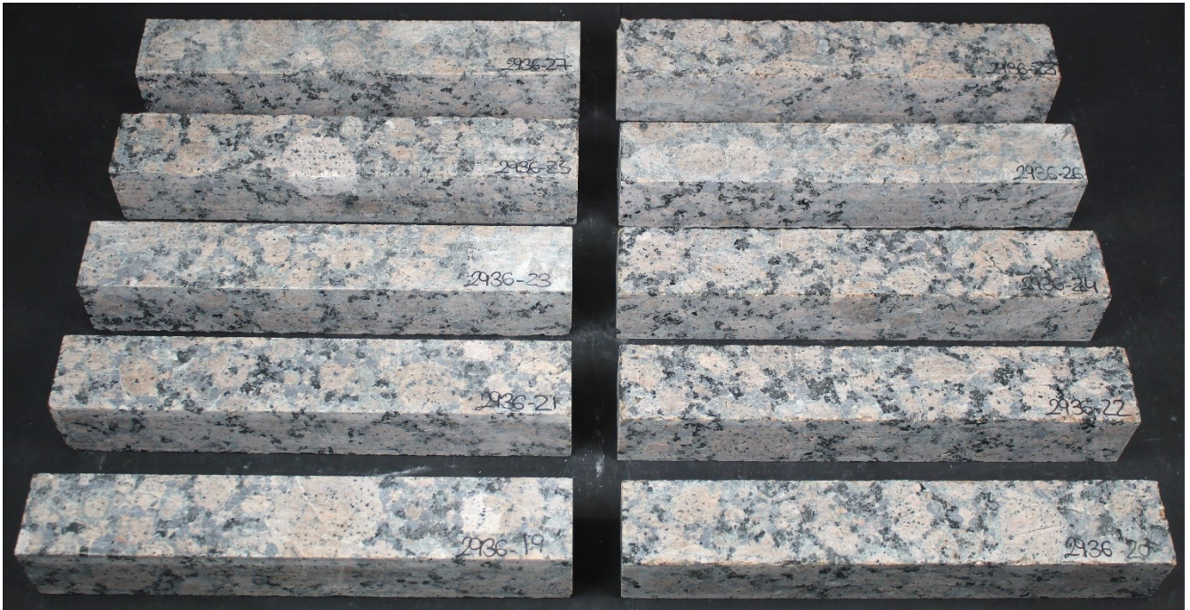
Set 2 after 56 freeze-thaw cycles
