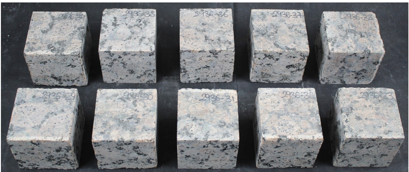
Set 2 after 56 freeze-thaw cycles
