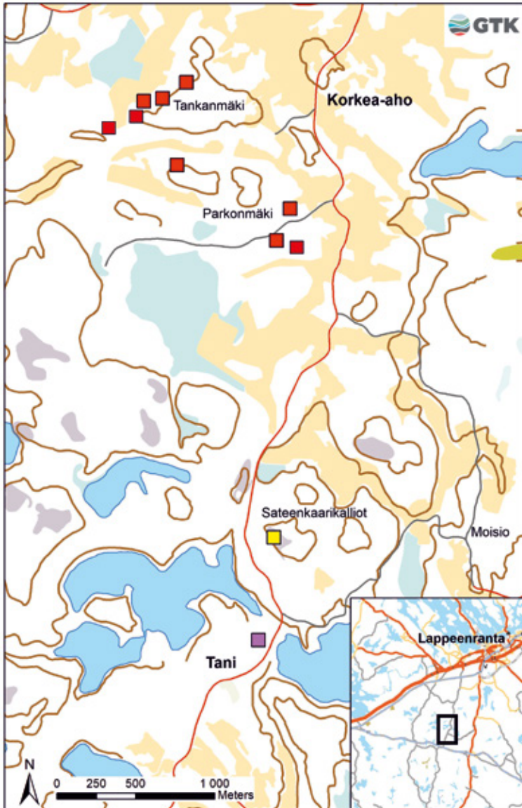
Figure 17. Location of the old quarries in the villages of Tani and Korkea-aho. Red squares: even-grained hornblende rapakivi granite (the Lappee granite). Yellow square: porphyritic granodiorite. Purple square: even-grained biotite rapakivi granite (the Tani granite). © National Land Survey of Finland.
