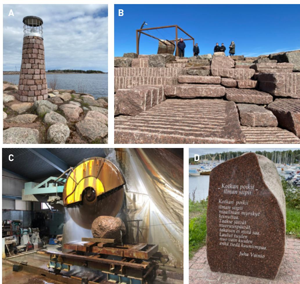
**Figure 11.** Examples of applications of natural stone along the Juha Vainion katu Street. A. Lighthouse made of recycled sett stones. B. Ramp into the sea prepared in leftover stone. C. Sawing of runestones in processing plant. D. Runestone with song text by the Kotka-born songwriter Juha Vainio. Photos A, C, D: Olavi Selonen, B: Heikki Palin.
