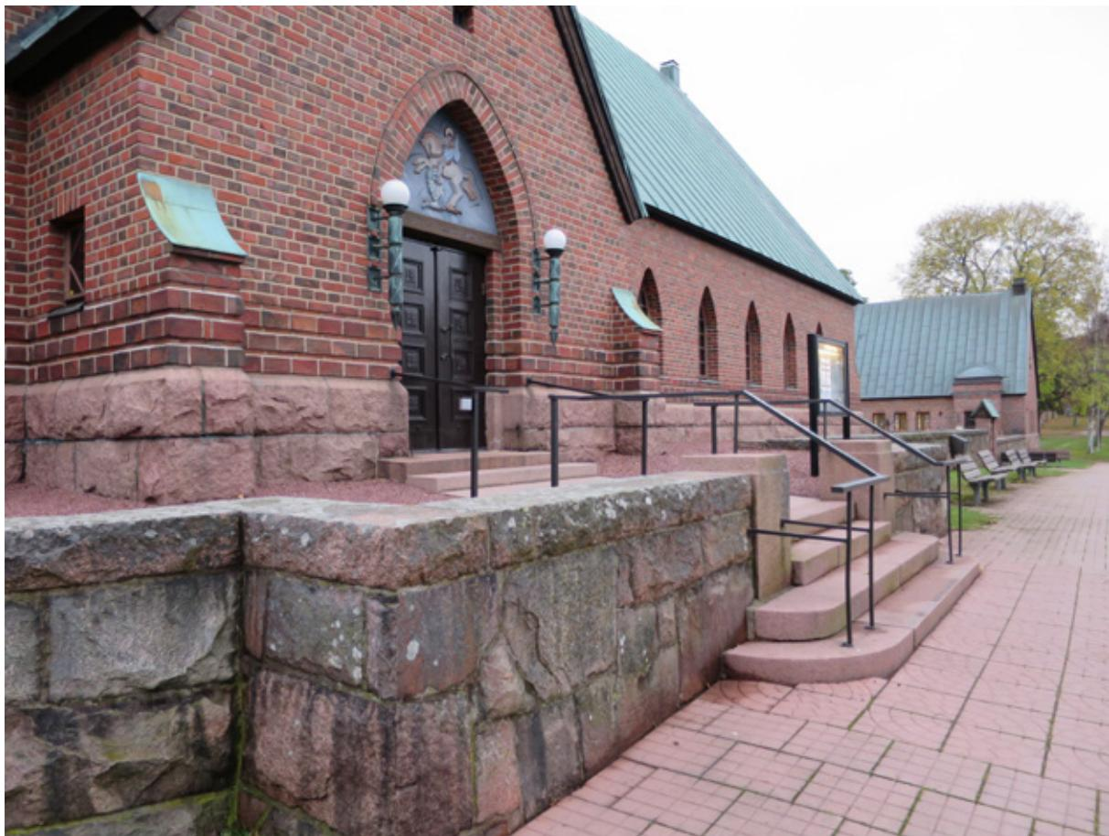
**Figure 13.** The foundation, masonry, and staircase of the Saint George's Church in Mariehamn is made of local red rapakivi granite. Photo: Olavi Selonen.
