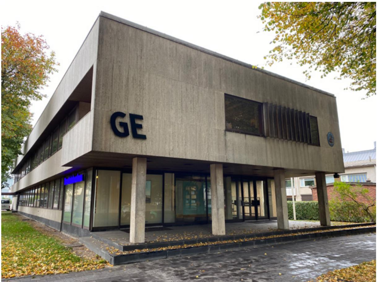
**Figure 14.** The façade of the GE office building in Mariehamn is built in travertine slabs. When exposed to impurities of the city environment, the light-coloured stone becomes dark with time. Photo: Olavi Selonen.
