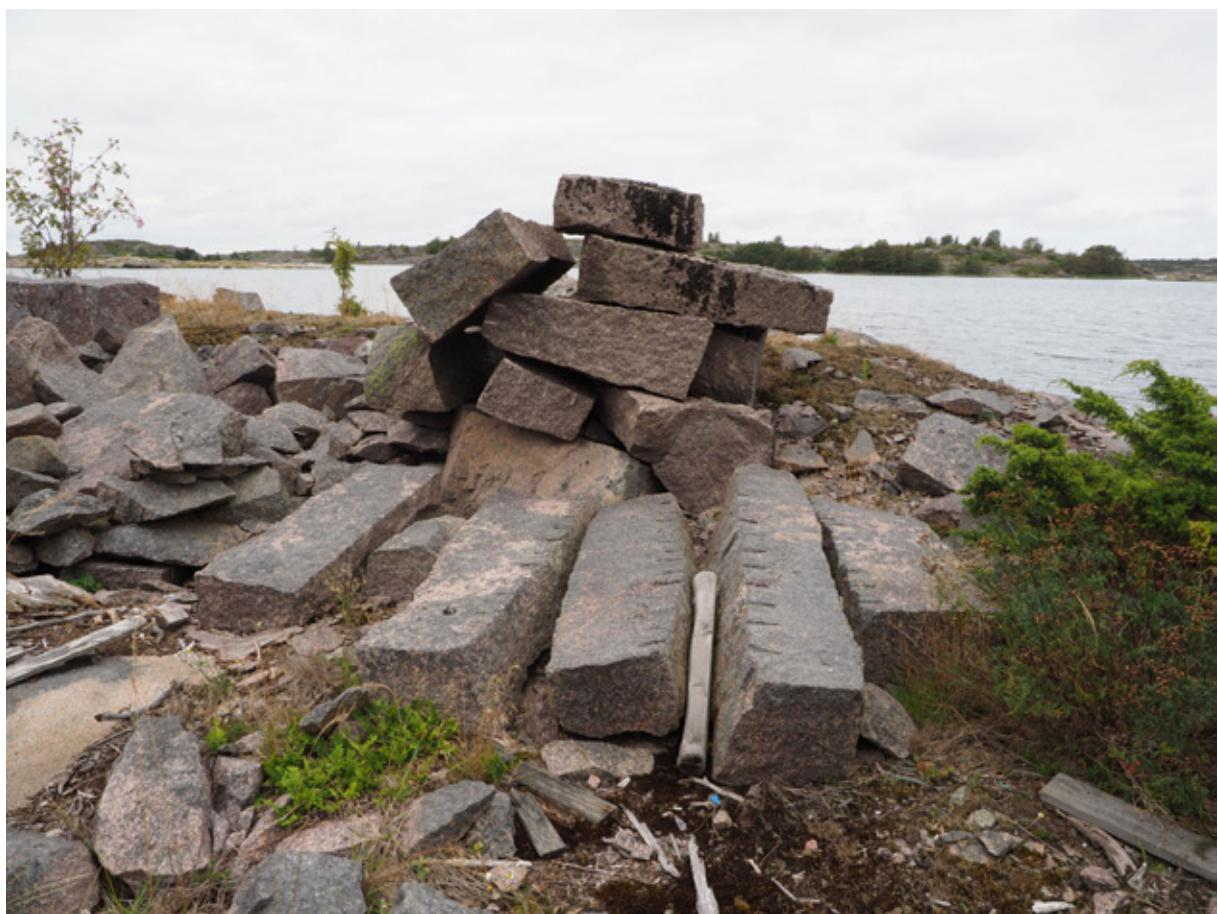
**Figure 7.** Short drill holes indicating good cleavability of Kökar granite. Photo: Carl Ehlers.
