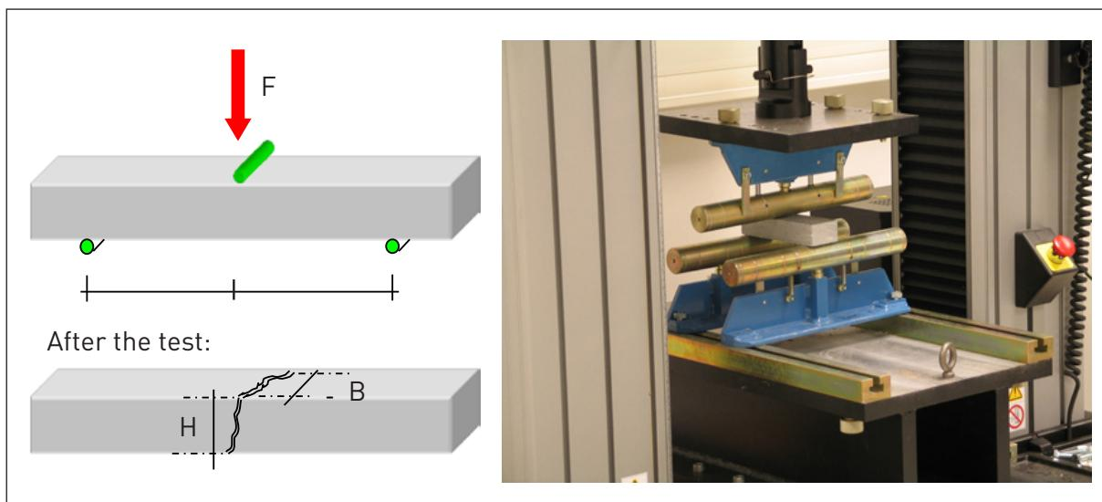
**Figure 1.** Determination of flexural strength under concentrated load according to the EN 12372.  $I$  = distance between the supporting rollers.  $F$  = load.  $B$  = width of the specimen adjacent to the plane of fracture.  $H$  = thickness of the specimen adjacent to the plane of fracture. The flexural strength  $R_{tf}$  is calculated as:  $3Fl/2Bh^2$  (MPa).
