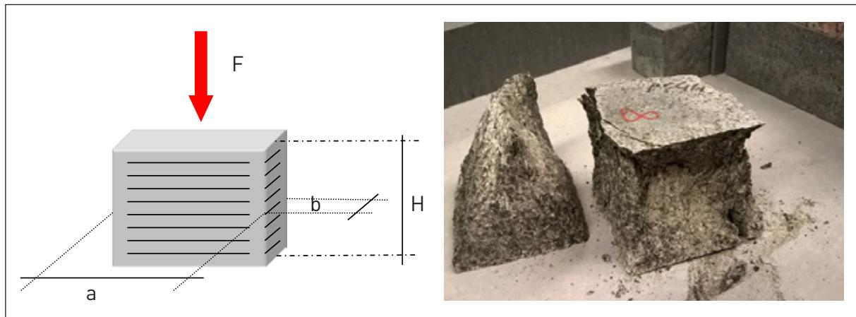
**Figure 2.** Determination of compressive strength according to the EN 1926.  $F$  = load.  $a$ ,  $b$ ,  $H$  = the three directions of measurement. The compressive strength  $R$  is calculated as:  $F/(a*b)$  (MPa).
