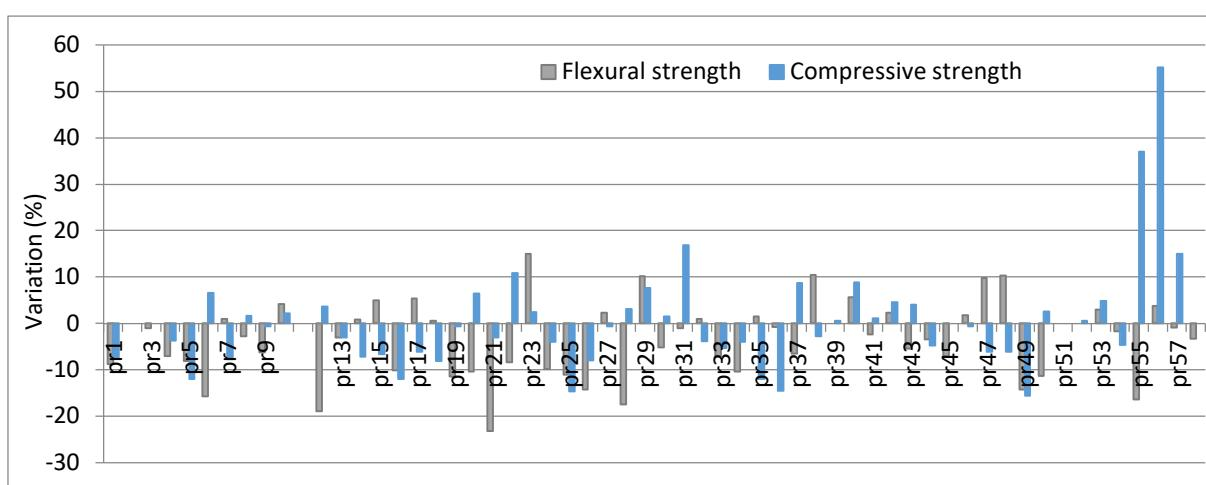
**Figure 8.** Percentage variation of flexural and compressive strength.
