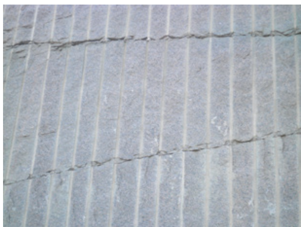
Figure 15. Deformation of the lower part of a horizontal sheet. Movements due to release of rock stress in the medium-grained porphyritic granite. Photo: Andrey Ivanov.
