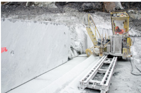
Figure 7. Quarrying of soapstone. Soapstone is quarried by sawing a horizontal and a vertical cut to form a ledge. The soapstone blocks are removed from the ledge with a wheel loader. Photo: Esko Koistinen.
