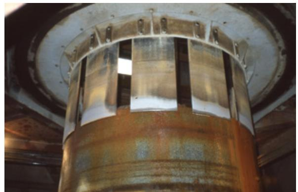
A rotating cylindrical saw was used for dressing of the surfaces of the granite roller. Photo: Roger Aapola.
