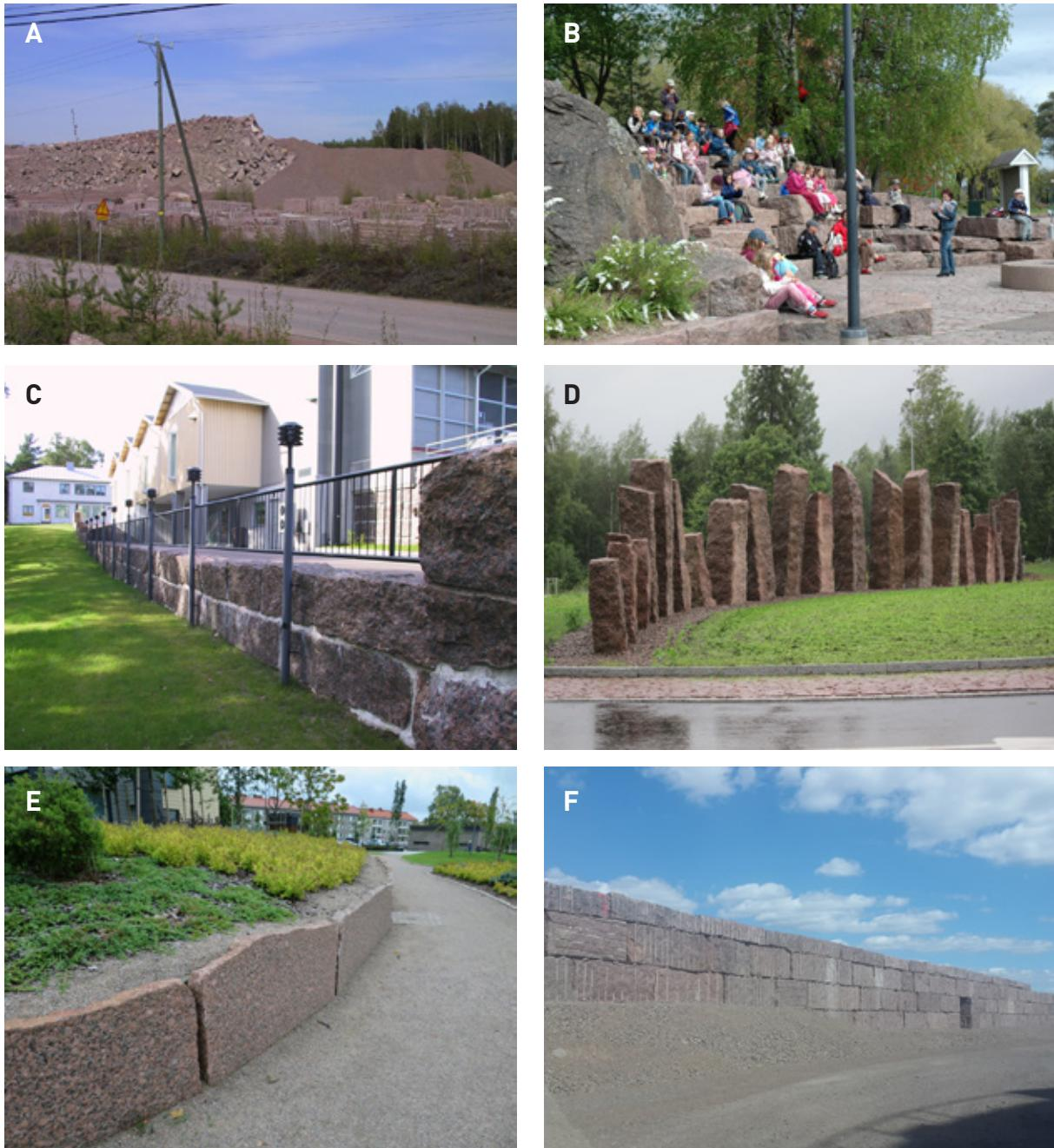
**Figure 10.** A selection of targets manufactured with leftover stone from the Wiborg batholith. A. Rock aggregate, Kotka. B. Benches, Sapokka Water Garden, Kotka. C. Wall, Virolahti. D. Monument, Kotka. E. Wall, Lappeenranta. F. Wall, Kotka. Photos: A, E: Olavi Selonen, B: Anne Vilkki-Lanu, C: Palin Granit Oy, D: Paavo Härmä, F: Linjaporaus Lehtinen Oy.
