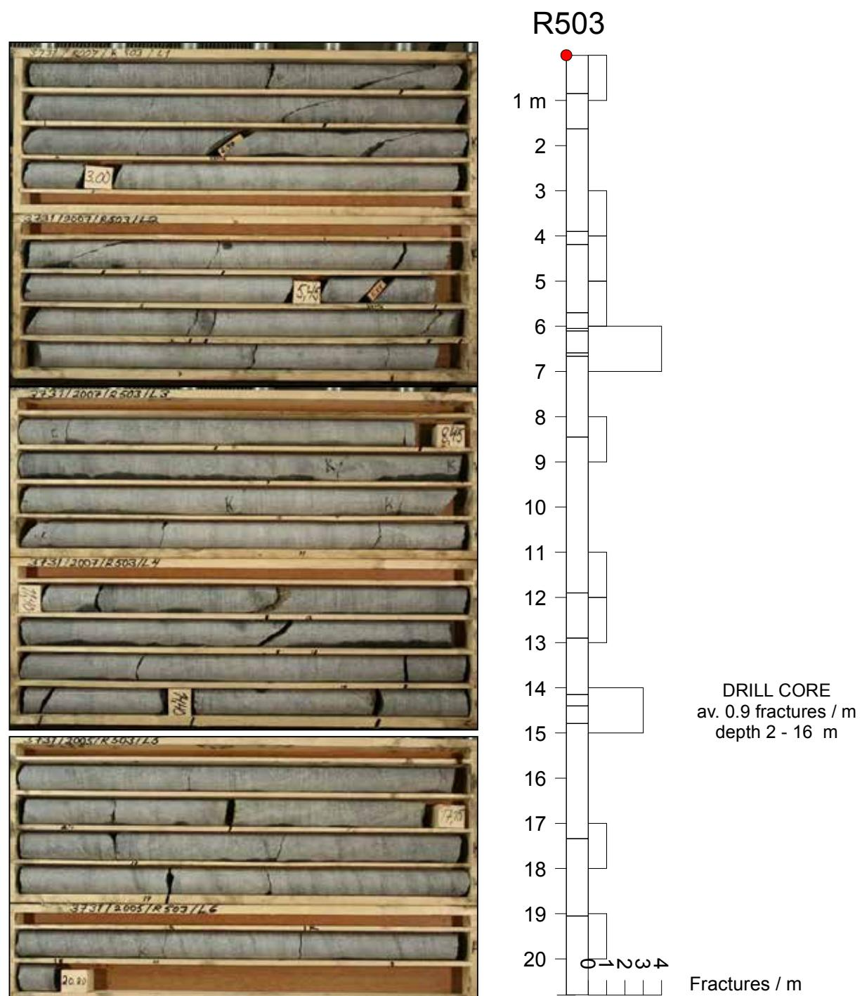
**Appendix 5.** A fracture histogram showing the fracture density defined from the video monitoring and from the drill core. Drill core R503.
