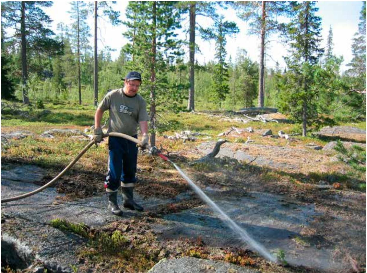
**Figure 3.** Washing of the outcrop surface. Photo: Risto Vartiainen.
