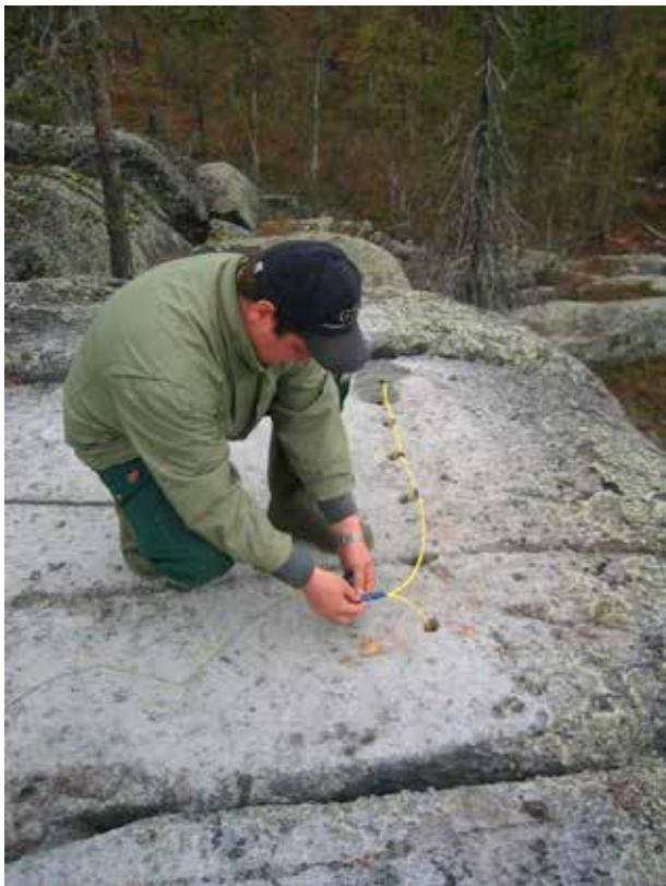
**Figure 4.** Sampling by blasting. Photo: Risto Vartiainen.
