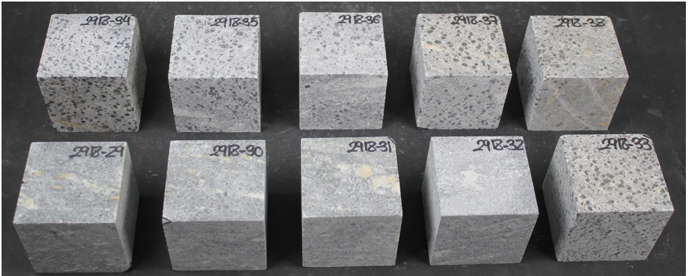
Set 2 after 56 freeze-thaw cycles
