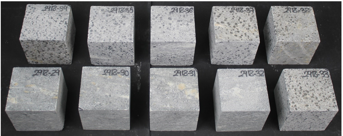
Set 2 after 56 freeze-thaw cycles
