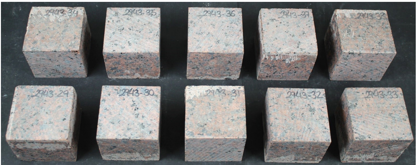
Set 2 after 56 freeze-thaw cycles
