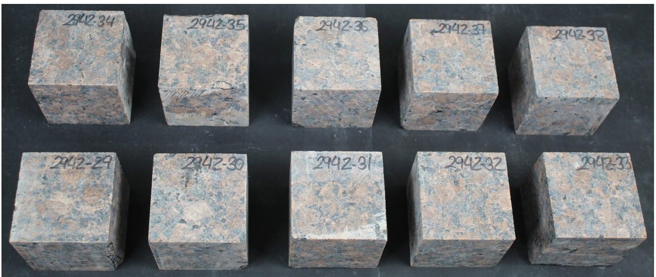
Set 2 after 56 freeze-thaw cycles
