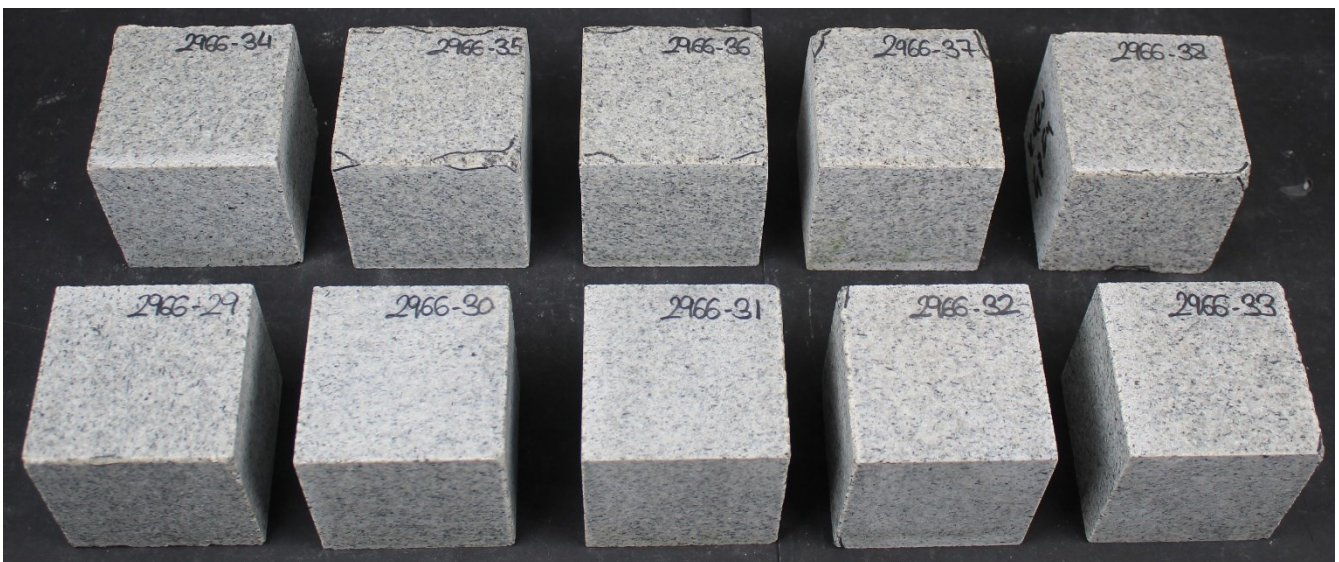
Set 2 after 56 freeze-thaw cycles
